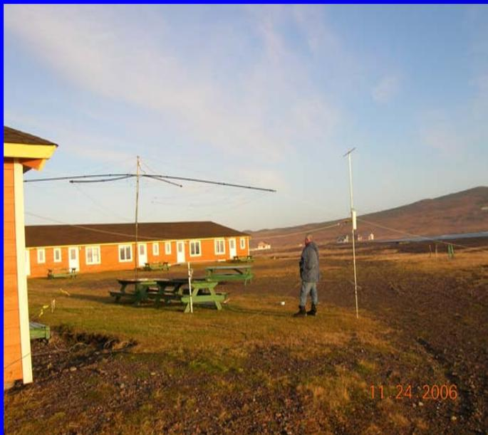
**The mast was 38 ft tall and supported our 160M inverted V, the 30M/15M inverted V and the Yankee Clipper special 80M “C”. The shorter mast had a 40M inverted V .**
